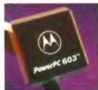
The 603 is Motorola's second generation RISC-based PowerPC processor.
